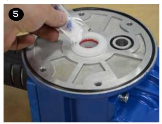
• Push the shaft (item 33) through the center of the shaft bushing (item 30). It is normal for this to be a tight fit, especially if the shaft and shaft o-rings (item 31) are in good condition.
