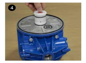
S Inspect the shaft (item 33) for damage. It is common for shafts to become grooved during service. Grooving is normally caused by carbonized oil and/or abrasive foreign material getting trapped between the seal and the shaft. Over time, deep grooves can form in the shaft. When that occurs, it is recommended that the shaft be replaced.
