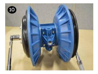
Install the liquid chambers (item 19) by placing one side over the diaphragm. Start all bolts & nuts (items 16, 18, 28) before tightening and torqueing. Torque all fasteners in a star pattern. Repeat to install the second liquid chamber. Ensure both chambers are orientated the same and that the inlet and outlet ports are vertical when facing the front of the pump as shown.
