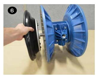
To remove the remaining diaphragm(s) (items 21/22) and plates (items 20 & 23) from the shaft (item 33), place the shaft in a vise. Using a 6-sided 32 mm wrench, remove the remaining diaphragm(s) and plates.
