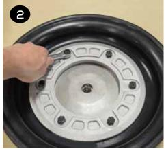
B Place the bump stop (item 32) onto Apply a couple drops of a medium strength thread locker, such as Loctite® 246, to the threads on end of shaft. Thread the shaft (item 33) into the outer plate (item 20) until it is snug.
