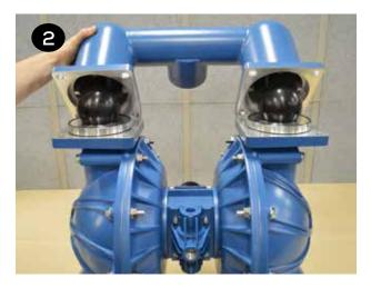
Repeat the above steps for the suction manifold (item12). The seat o-rings, valve seats and valve balls (items 13, 14, & 15) are located in the liquid chambers (item 19).
