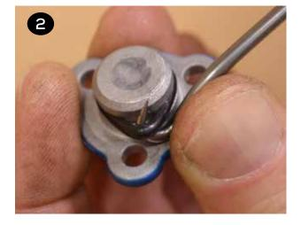
Remove the valve body (item 3) by removing the (4) socket head cap screws and washers (items 1 & 2) that attach the valve body to the muffler plate (item 38) with a 6 mm hex wrench Pull the valve body and gasket (items 3 & 37) off the front of the center section (item 36) and the muffler plate gasket, muffler plate and muffler (items 38, 39, & 41) off the back.
