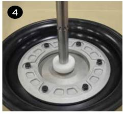
• The shaft (item 33) and shaft o-rings (item 31) should retain the lubricant that was factory applied. If they appear dry, apply a light coat of lithium thickened grease. Avoid over-lubrication as it can cause decreased performance of the air distribution system.
