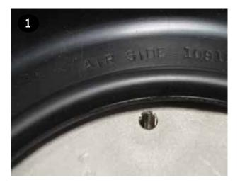
Place the inner plate (item 23) on the diaphragm. Ensure the round recess one end of the shaft (item 33). in the plate faces the diaphragm (item 22). Tighten the (6) bolts (items 24, 25, & 26) in a star pattern using a 13 mm wrench.
