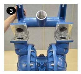
• Remove both liquid chambers (item 19) by removing the (10) bolts & nuts (item 16, 18, & 28) on each liquid chamber using a 16 mm wrench. Inspect and replace diaphragms if needed. • To remove the diaphragms (items 21/22), begin by loosening the (2) outer plates (item 20) using two 32 mm wrenches.
