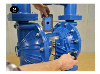
• Place the new gasket (item 37) on the air valve (item 3) and ensure the slots in the gasket align with the slots in the air valve and valve plate (item 10).
